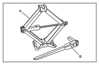
The tools to be used are the jack (A) and the wheel wrench (B).
